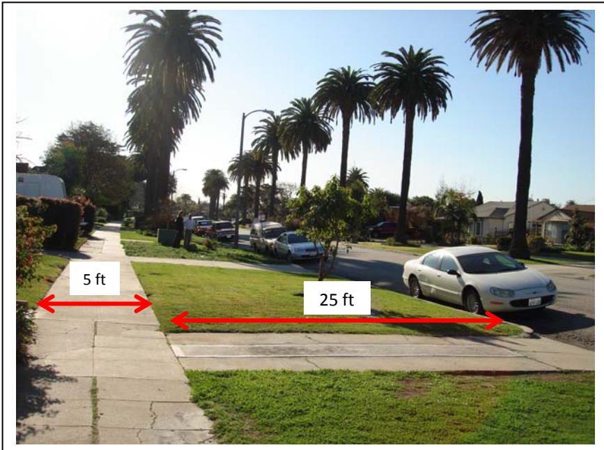
Figure A2. Typical configuration of sidewalk, driveway, grassy area, and paved street
